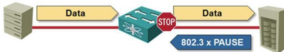
The switch stops sending data to the storage array after receiving the PAUSE frame, causing the data sent by the server to accumulate in the switch's internal buffers until the switch has to tell the server to cease transmitting data by sending its own PAUSE frame.
