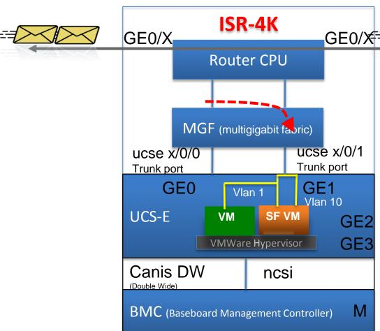
On the ISR-4K, the replicated traffic can be sent to SourceFire Virtual Sensor using either UCSEx/0/0 interface or UCSEx/0/1 interface, both interfaces can be configured as trunk ports
