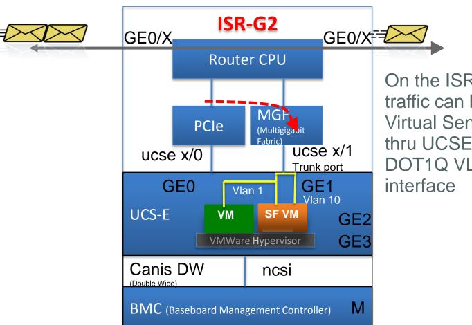
On the ISR-G2, the replicated traffic can be sent to SourceFire Virtual Sensor as untagged traffic thru UCSEx/0 interface or as DOT1Q VLAN on UCSEx/1 interface
