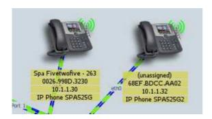
Navigate to the CCA Configuration drawer to 'Users and Extensions' and notice CCA discovered the proper phone type (G is different from G2 so don't overwrite that) and see that "NoInfo" for name, number, voicemail ...etc., is shown for the unassigned G2 phone, which you then EDIT.
