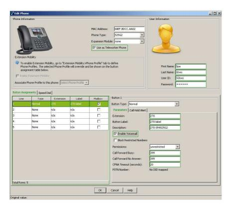
Lets check the SPA525G and make sure we check the box for Teleworker Phone (this places MTP on its ephone).
