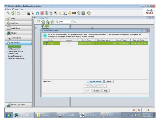
4.- The next windows is the "Upgrade Settings" where we can to upgrade the device, the system software, the IOS and CUE, we select the CUE option and appear the CUE window upgrade options.
