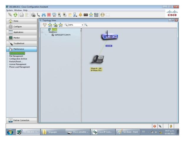
3.- A window will appear, where we list the devices that have, in my case is a UC540, device type, current version. And the down part a button named "Upgrade Settings".
