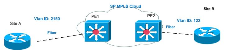
The incoming frame from site A is tagged with vlan 2150. We need PE1 to remove the vlan tag of 2150 and forward the frame to PE2. the frame should reach PE2 with no tag then in the egress port it's encapsulated with vlan tag 123 to be transported to Site B
