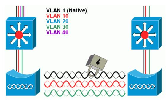
In order to encrypt data that passes over the radio link, apply encryption to only the SSID of the Native VLAN. That encryption applies to all other VLANs. When you bridge, there is no need to associate a separate SSID with each VLAN. VLAN configurations is the same on both the root and non-root bridges.
