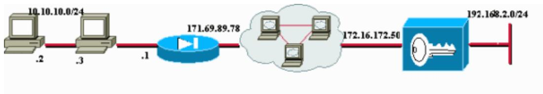
There are VPN Clients on the two PCs (10.10.10.2 and 10.10.10.3) behind the PIX Firewall. The PIX in this scenario is simply being used as a PAT device, and conducts PAT on these addresses to 171.69.89.78. Any device that is able to PAT multiple internal connections can be used here. The VPN 3000 Concentrator public address is 172.16.172.50. The following example demonstrates how to configure the clients and the concentrator so that NAT-T is used during the IKE negotiation.
