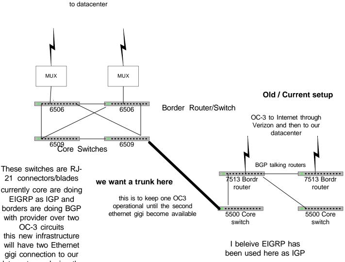
with provider over two OC-3 circuits this new infrastructure will have two Ethernet gigi connection to our datacenter replacing the OC-3 circuits but since one Ethernet gigi won't become available, they need to keep the old infrastruture in place and use one of the OC3s until the second Ether gig circuit arrives
