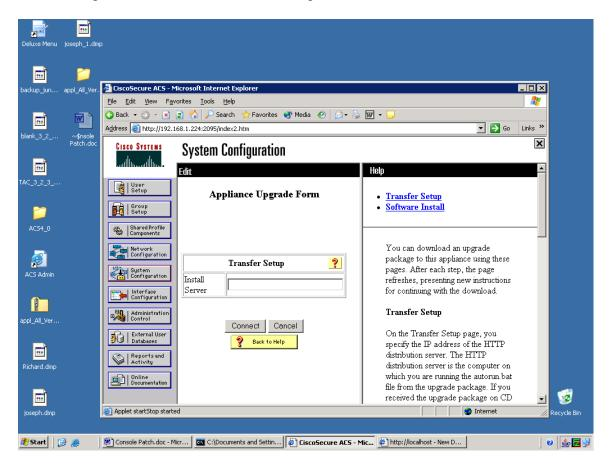
Provide in ip address of system from where we are applying this patch, in our case our desktop ip address, then click connect.
