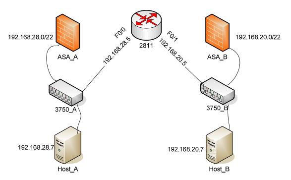
Using IP 192.168.28.7 gateway 20.1 user can ping but can not access the other network like telnet etc.
