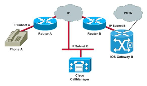
Subnets A and B can both reach Subnet X. Subnet X can reach Subnets A and B. This allows the establishment of TCP connections between the end stations (A and B) and the Cisco CallManager. Therefore, signaling can reach both end stations without any problems, which allows the establishment of calls between A and B.
