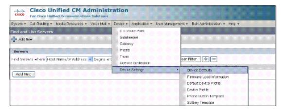
**Note:** In order to get the phone load name from CallManager 4.x, go to **System > Device Defaults > Device Defaults Configuration** and copy the load information.
