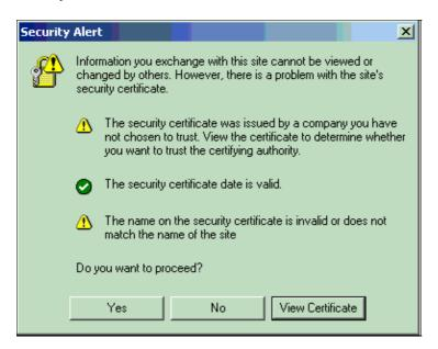
Users are prompted to accept the certificate from the WLC because the clients do not have a trusted root certificate for the certificate that is installed on the WLC. The SSL certificate on the WLC is not in the list of certificates that the client system trusts. There are two ways to stop the generation of this web-browser security alert popup window:
