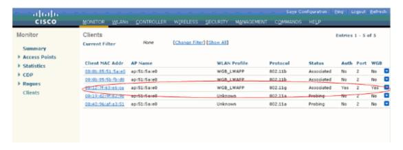
Click the MAC address of the desired client in order to view the details of the WGB. The Clients > Detail page appears.
