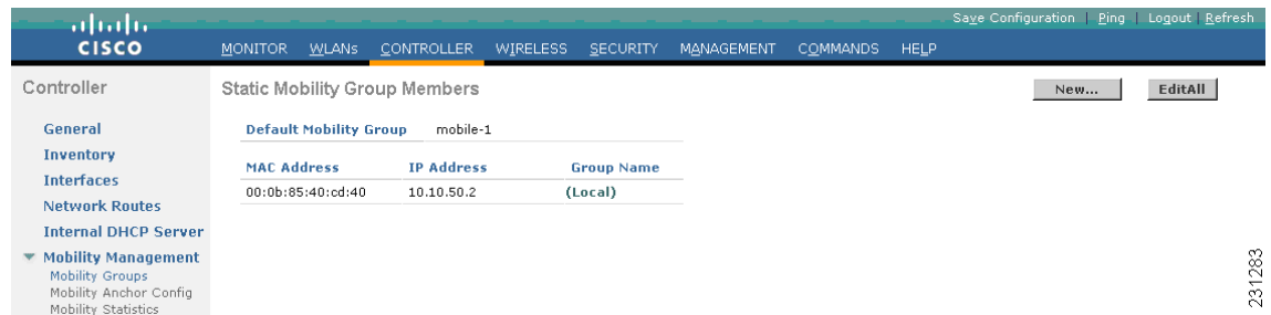
Figure 16 Controller > Static Mobility Group Members Window
