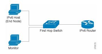
A separate and independent instance of IPv6 First Hop Security runs on each VLAN on which the feature is enabled.
