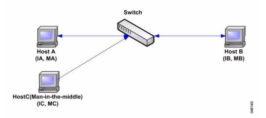
Hosts A, B, and C are connected to the switch on interfaces A, B and C, all of which are on the same subnet. Their IP, MAC addresses are shown in parentheses; for example, Host A uses IP address IA and MAC address MA. When Host A needs to communicate with Host B at the IP layer, it broadcasts an ARP request for the MAC address associated with IP address IB. Host B responds with an ARP reply. The switch and Host A update their ARP cache with the MAC and IP of Host B.
