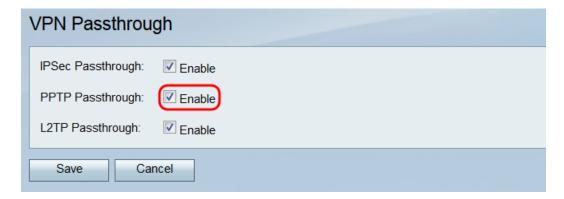
Step 4. In the *L2TP Passthrough* field, the **Enable** check box is checked by default. L2TP (Layer 2 Tunneling Protocol) is a tunneling protocol used to transmit PPP packets in VPNs. If you do not want any L2TP traffic to pass through the device, uncheck this box.
