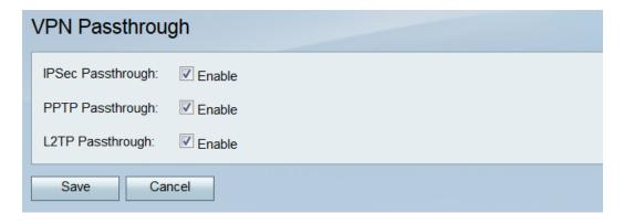
Step 2. In the *IPSec Passthrough* field, the **Enable** check box is checked by default. IPSec (Internet Protocol Security) is a suite of protocols that allows secure exchange of packets. If you do not want any IPSec traffic to pass through the device, uncheck this check box.
