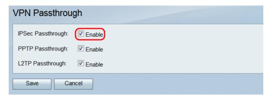
Step 3. In the *PPTP Passthrough* field, the **Enable** check box is checked by default. PPTP (Point-to-Point Tunneling Protocol) is a way to transmit PPP (Point-to-Point Protocol) packets over a VPN. If you do not want any PPTP traffic to pass through the device, uncheck this box.
