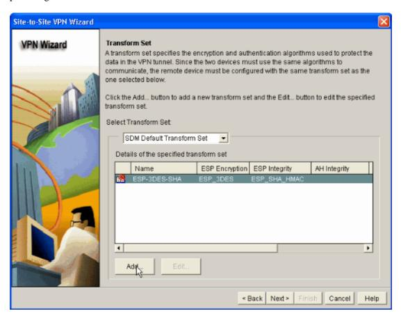
11. Provide the **Transform Set** details (**Encryption and Authentication Algorithm**) and click **OK** as shown.
