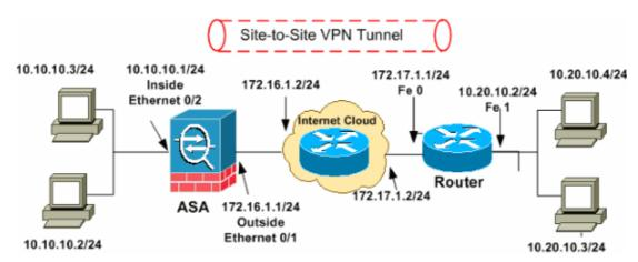
**Note:** The IP addressing schemes used in this configuration are not legally routable on the Internet. They are RFC 1918 addresses, which have been used in a lab environment.
