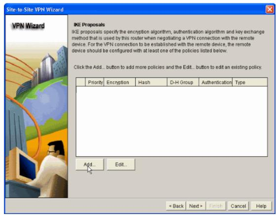
8. Provide Encryption Algorithm, Authentication Algorithm and the Key Exchange method as shown here, then click OK. The Encryption Algorithm, Authentication Algorithm and the Key Exchange method values should match with the data provided in the ASA.
