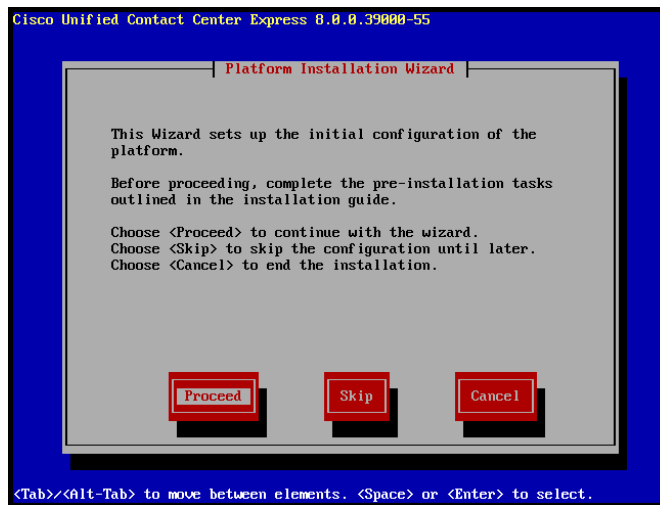
Figure 3 Platform Installation Wizard Window
