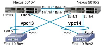
**Note:** HPVC Flex-10 supports LACP, so configure the Nexus 5000 interfaces to channel-group mode "active" that are connected to the Flex-10 in the Port-Channel
