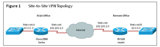
A site-to-site IPsec VPN tunnel is configured and established between the Cisco RV320 Gigabit Dual WAN VPN Router at the Remote Office and the Cisco 2900 Series ISR at the Main Office.
